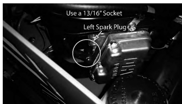
Spark Plug Component and Details
